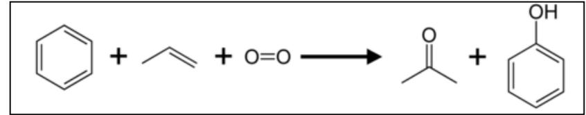
Figure 5: Hock process for producing phenol<sup>[21]</sup>
