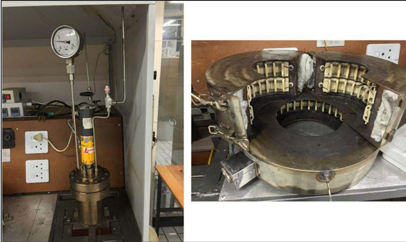
Figure 6: Batch HTL reactor (left) and removable heating jacket (right)
